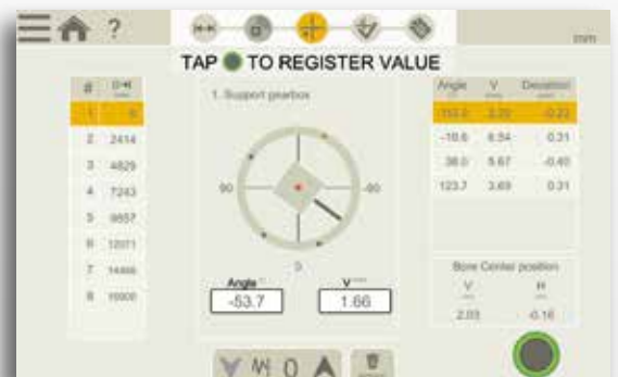
Bore center measurement view. Measure from 3 to 50 points at each bore position in Multipoint measure mode. Remeasure any point at any stage.
