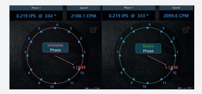
Moreover, incorporating a real-time stability indicator is critical in this process. This feature assesses the consistency of the phase measurements over time.
