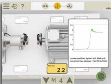
Soft Foot check on both machines.
