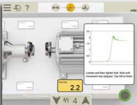
Soft Foot check on both machines.
