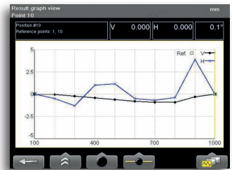
Straightness program. Result graph.
