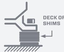
Dirt, grease, paint, or rust, between foot and base.
