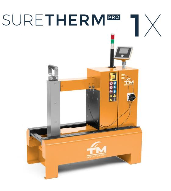
The new heating method, easy set on a modern touch screen, is specially developed for the heating of gears and bearings. The user can set the temperature and time (ramp), or place two sensors. The major advantage this provides is the temperature differential between the internal and external component materials remains low thus reducing the potential for material stress accumulation and subsequent potential distortional damage.
